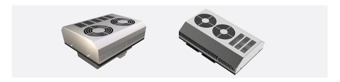
The thermoelectric cooling units PK 150-PS and PK 300-PS have a wide-range voltage input of 100-240 V. The power supply is integrated in these devises. The protected power supply is located on the outside of the cooler and thus outside the cabinet to be cooled. It eliminates a heat source inside. This results in a simple and faster installation and less space in the housing.
